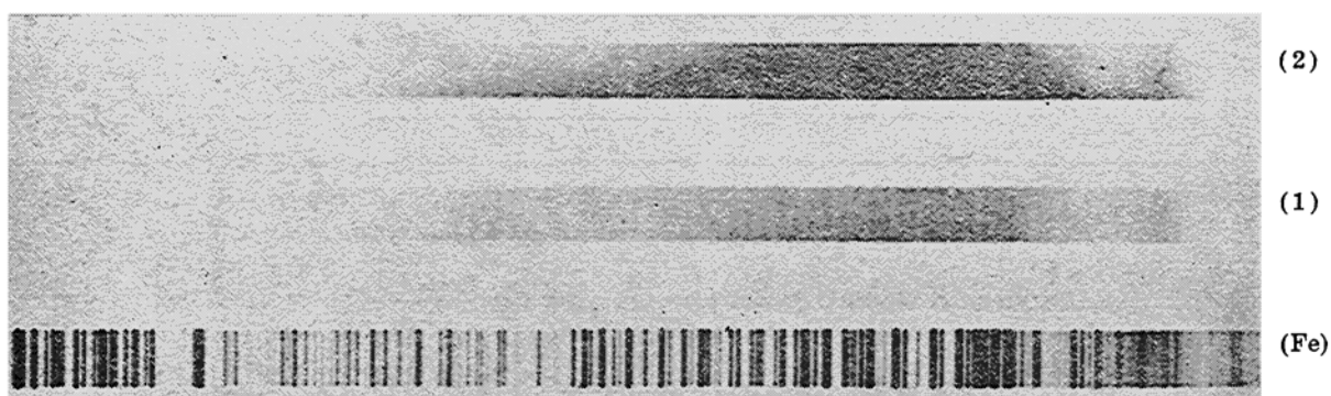
Fig. 3. Fluorescence spectra of (1) pure ZnS and (2) ZnS/Cu at +150^{\circ}\text{C} .
